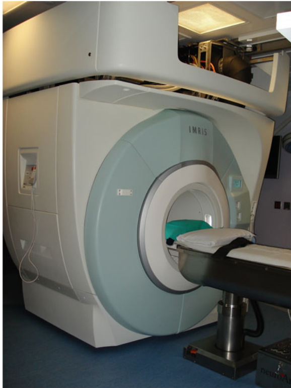
Fig. 3 IMRIS 1.5 T intraoperative magnetic resonance imaging system with the magnet suspended from ceiling rails. In the foreground is the MRI compatible surgical table
